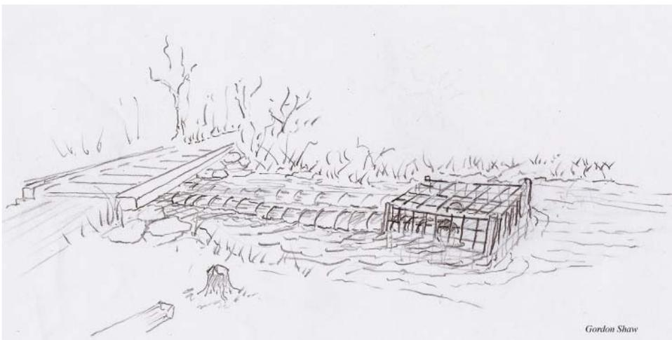
*Even if the beavers rebuild their dam under the bridge, the water can still flow through the pipes.*
